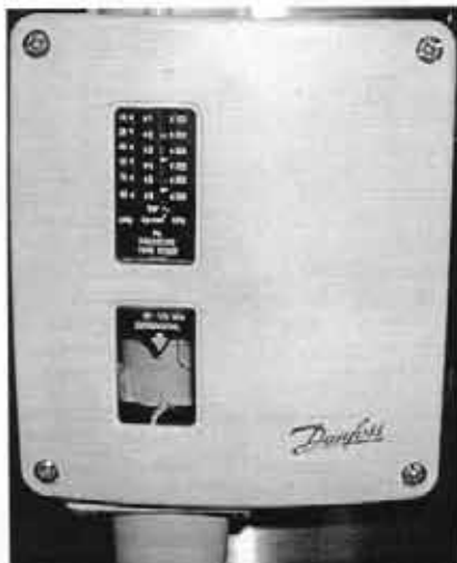
pressure regulator for jacket pressure
